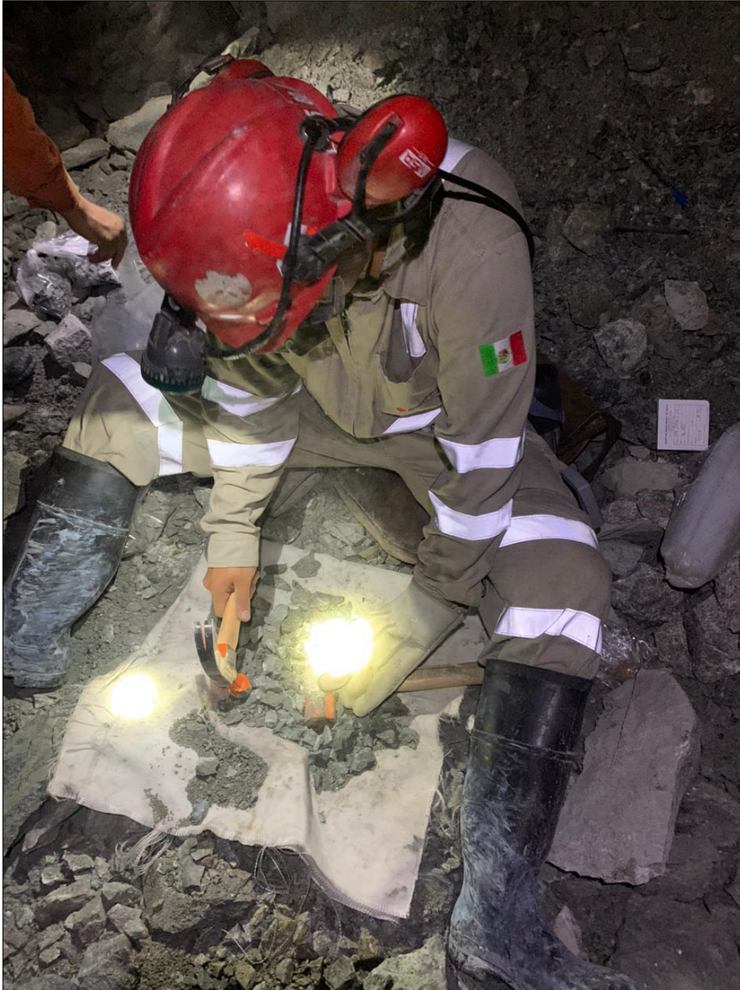
Figure 7-4: Homogenization Process of Sample Particle Size
