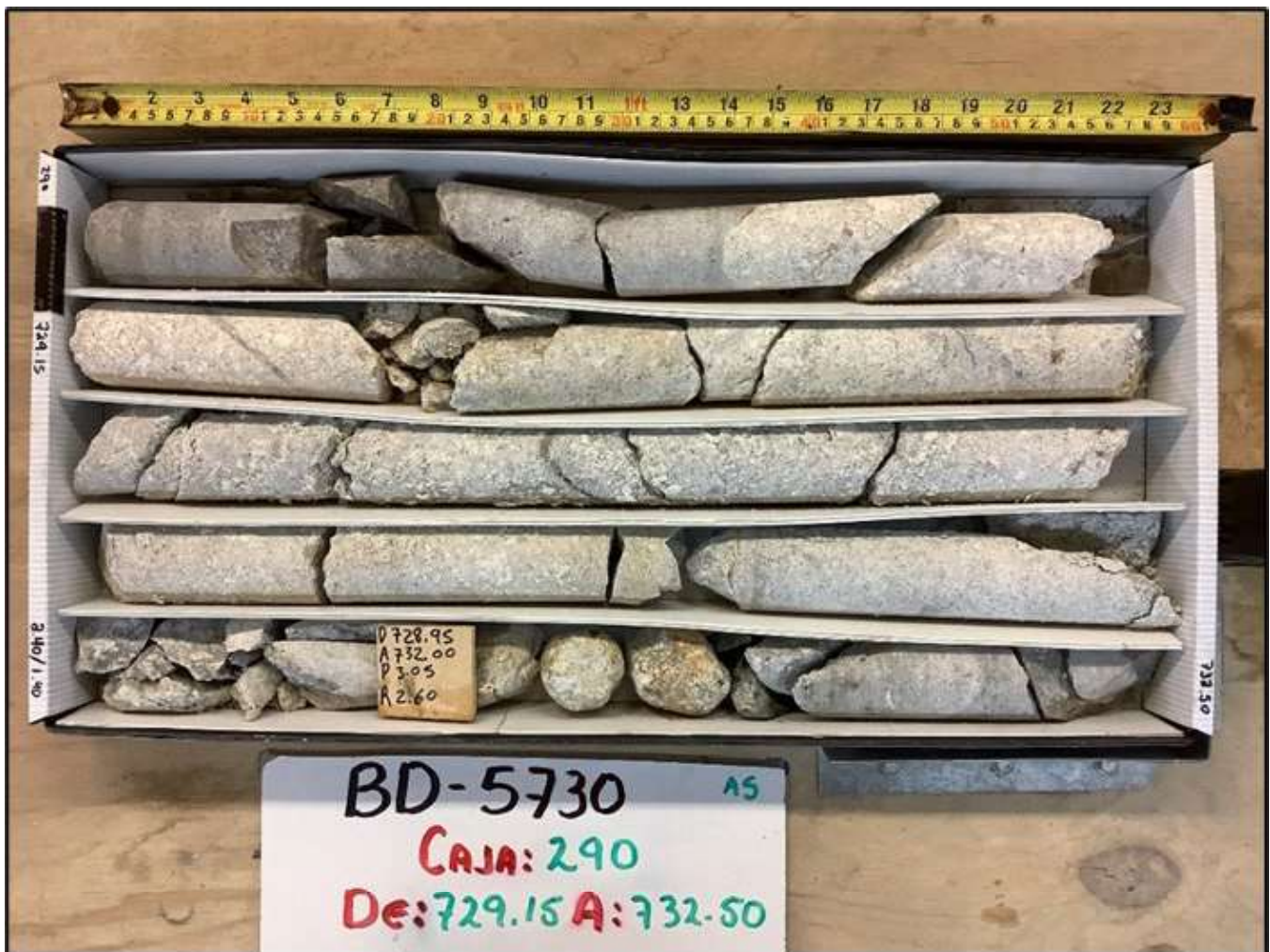
Figure 8.3: Example Core Box (BD-5730)
