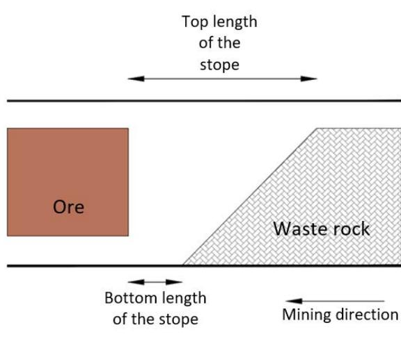
**Figure 13-18: Bench & fill longitudinal mining diagram**
