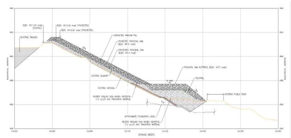
**Figure 15-7: Principal Dam cross section (after butress implementation)**
