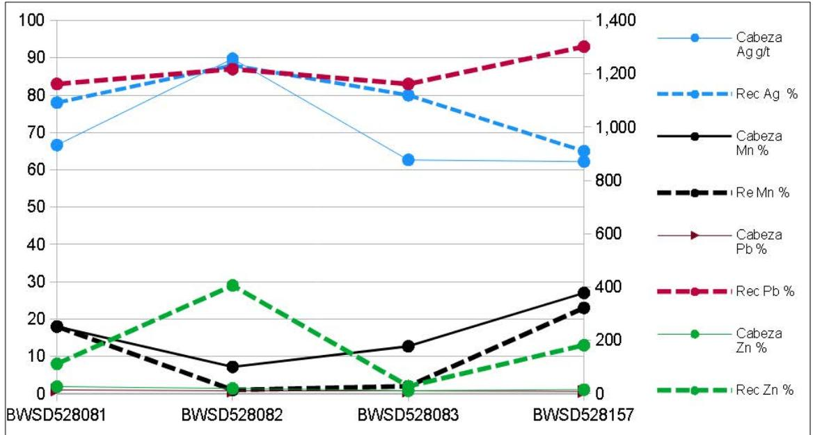
Figure 10-24: Tomasa testing, head grade and flotation recovery
