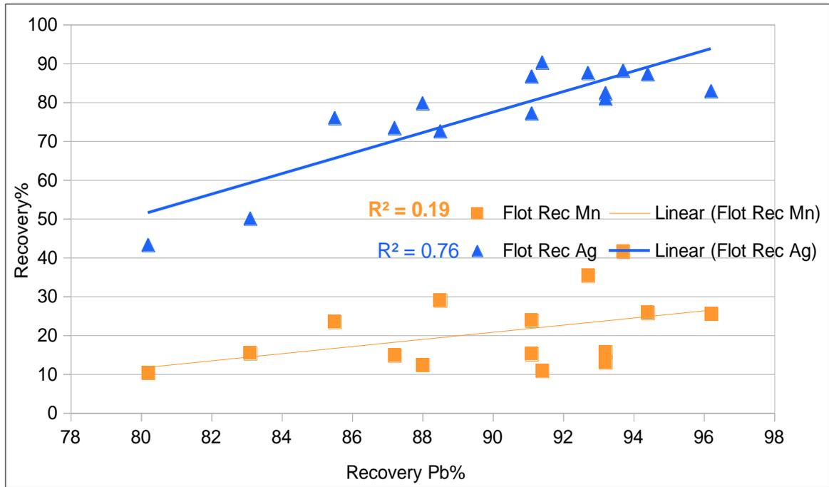
**Figure 10-15: Yumpag Testing, Recovery v/s Recovery Pb**
