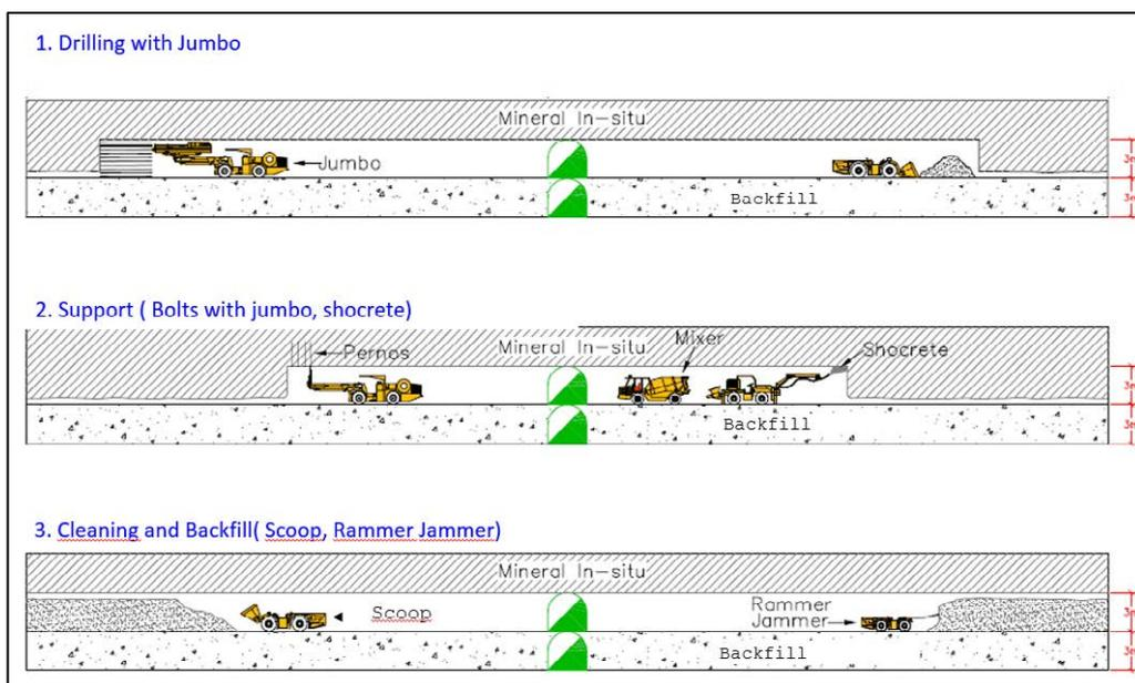
**Figure 13-9: OCF BM mining cycle**
