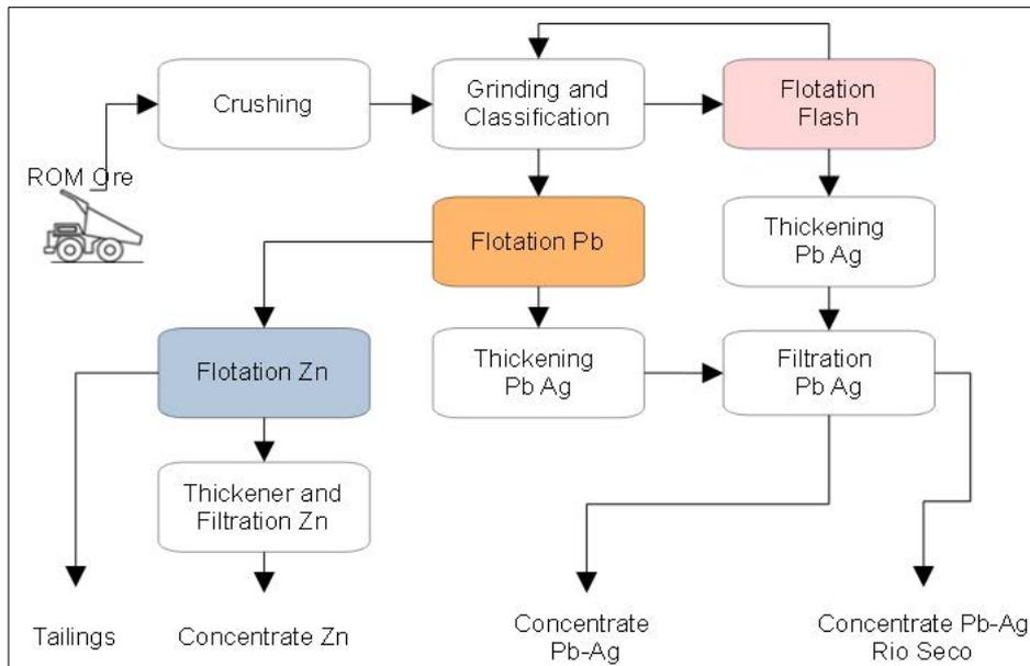
**Figure 14-7: Uchucchacua, Processing Circuit 2, Block Flow Diagram**
