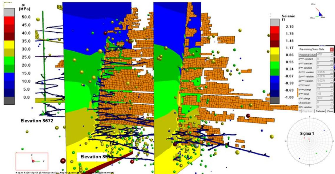
**Figure 13-17: Isovalues of induced stresses at Socorro mine**
