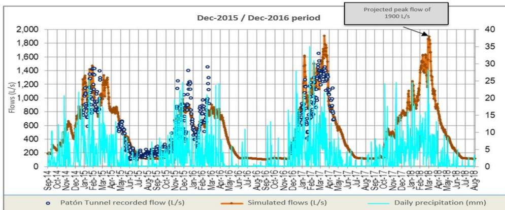
Figure 13-23: Paton tunnel discharge record (2014 - 2018)
