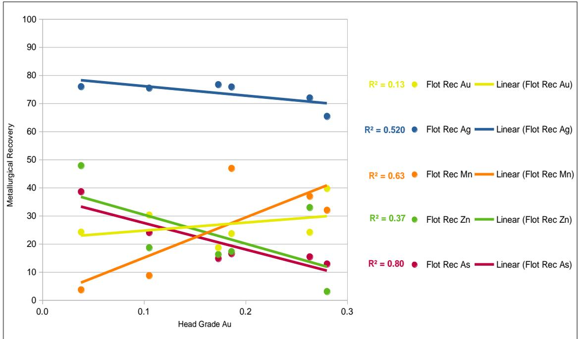
**Figure 10-5: Uchucchacua, Metallurgical Testing, Recovery v/s Head Grade Au g/t**
