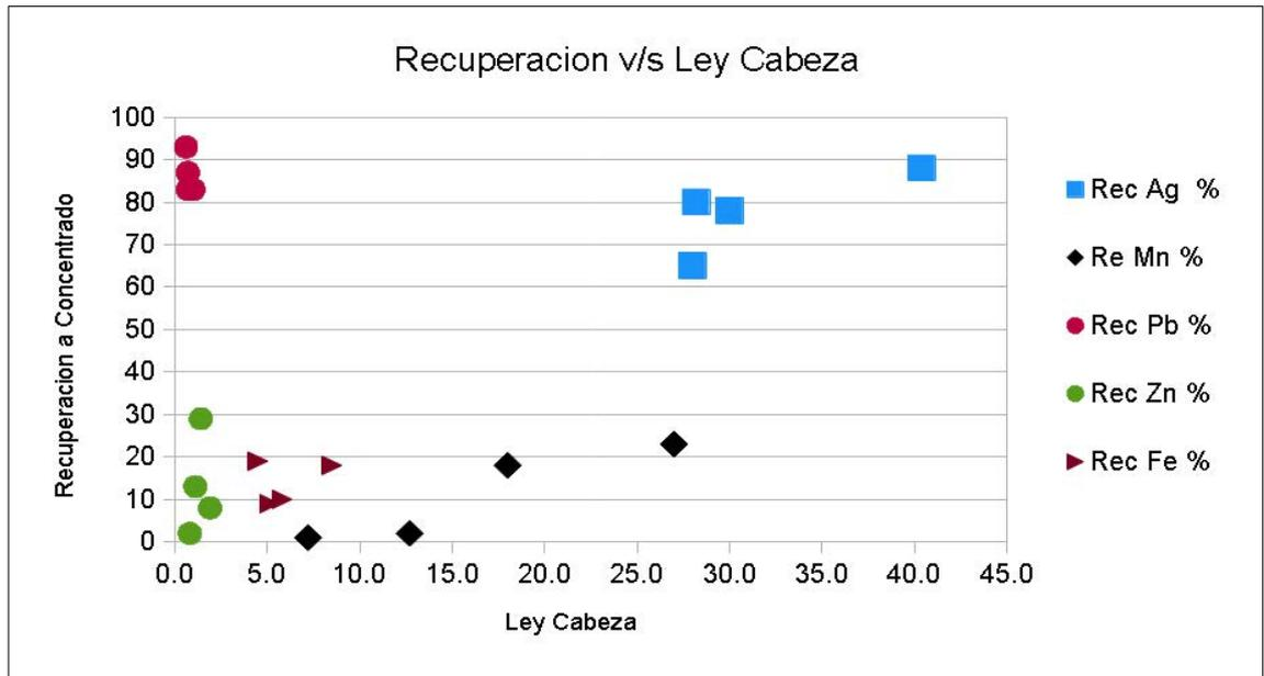
**Figure 10-25: Tomasa testing, flotation recovery versus head grade**
