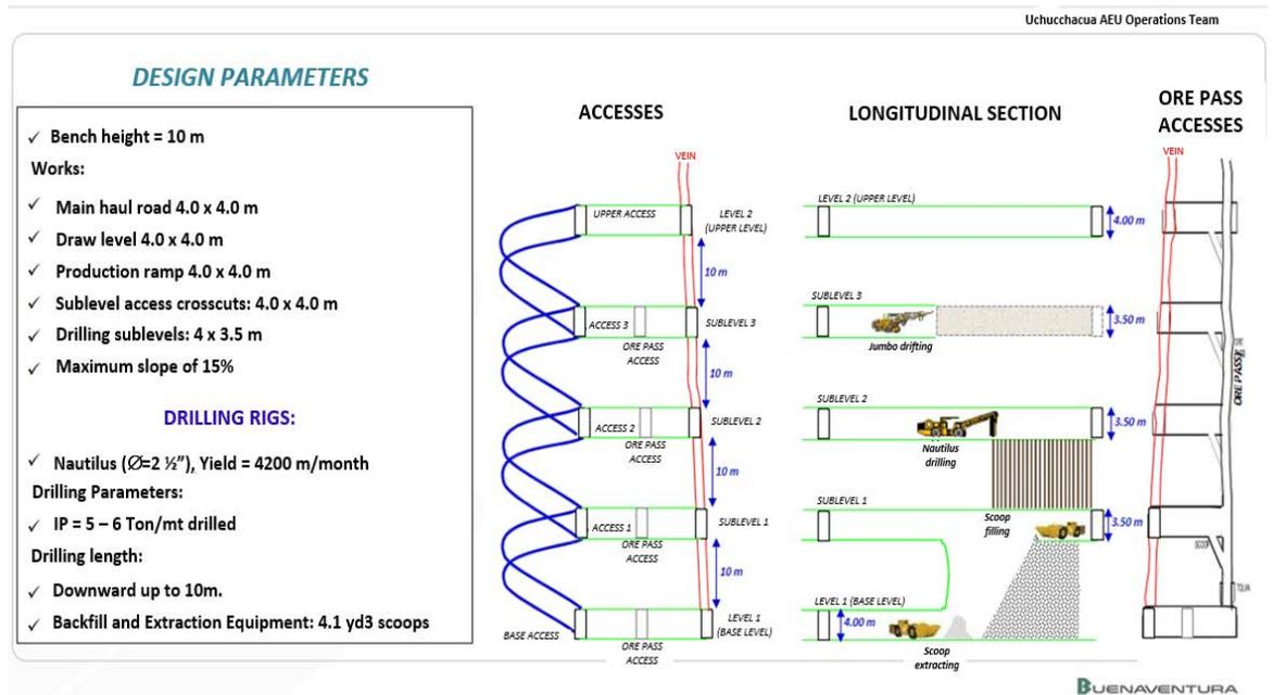
**Figure 13-5: Bench & Fill method at Uchucchacua: Sequence**
