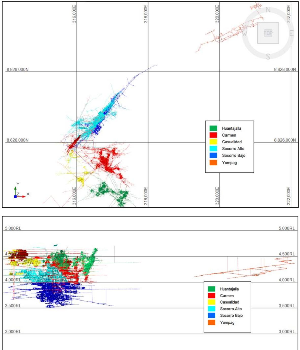
**Figure 13-30: Plan and isometric drawings of underground mines**
