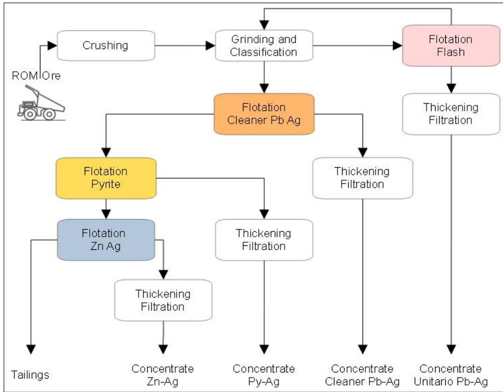
**Figure 14-5: Uchucchacua, Processing Circuit 1, Block Flow Diagram**
