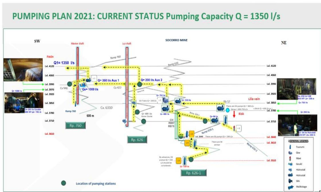
Figure 13-22: Current pumping system of Uchucchacua A.E.U.
